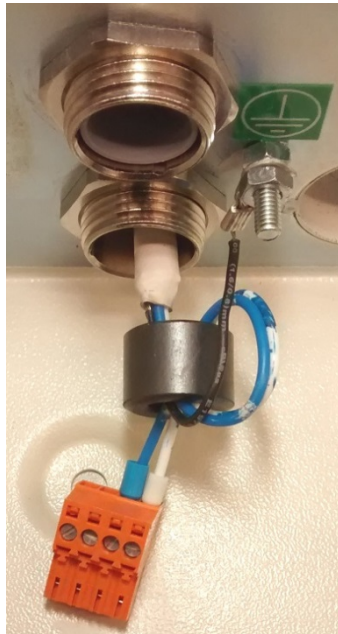
Figure 8: Looping relay connection wires around a suppression ferrite
